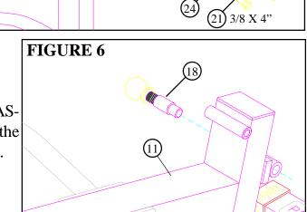
**STEP 8:**Securely assemble one 1/2" SPRING PIN AS-SEMBLY (18) into the spring pin barrel on the LEG FRAME (11) as shown in FIGURE 6.
